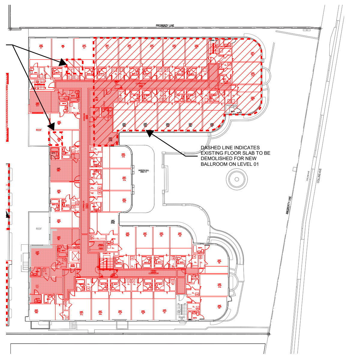
LEVEL 02: DEMOLITION PLAN
