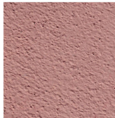
FINISH: LIGHT BROOM FINISH COLOR: MIAMI BEACH RED (CEMENT & MORTAR) PER PUBLIC WORKS DESIGN CONSTRUCTION STANDARDS
