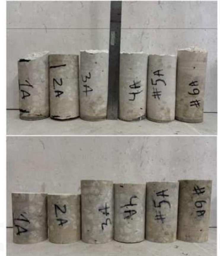
The Concrete compressive strength ranged from 1,480 to 2,560 PSI. Per Florida Building Code the concrete strength should be 5,000 PSI.
