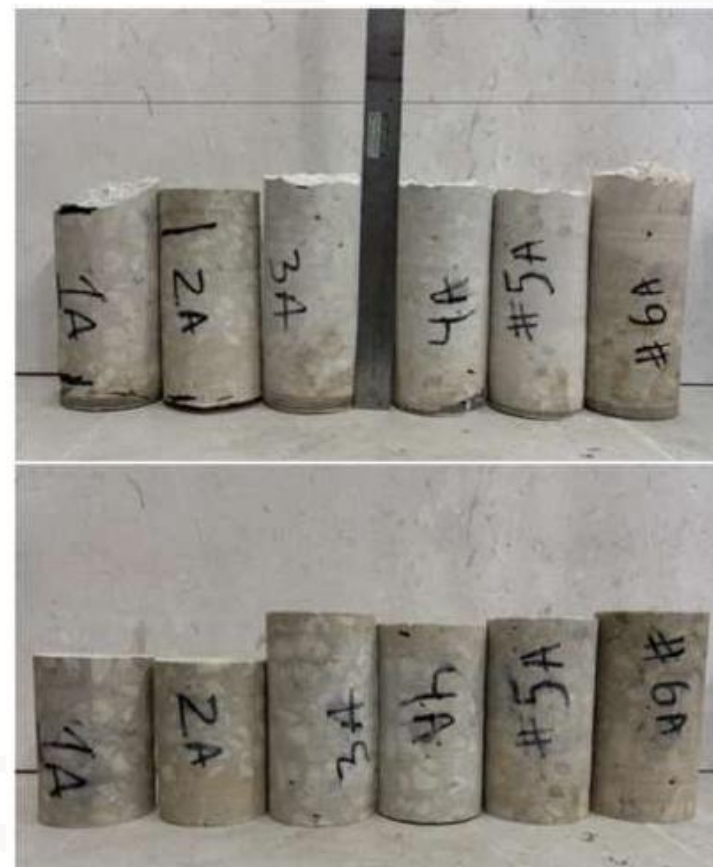
The Concrete compressive strength ranged from 1,480 to 2,560 PSI. Per Florida Building Code the concrete strength should be 5,000 PSI.
