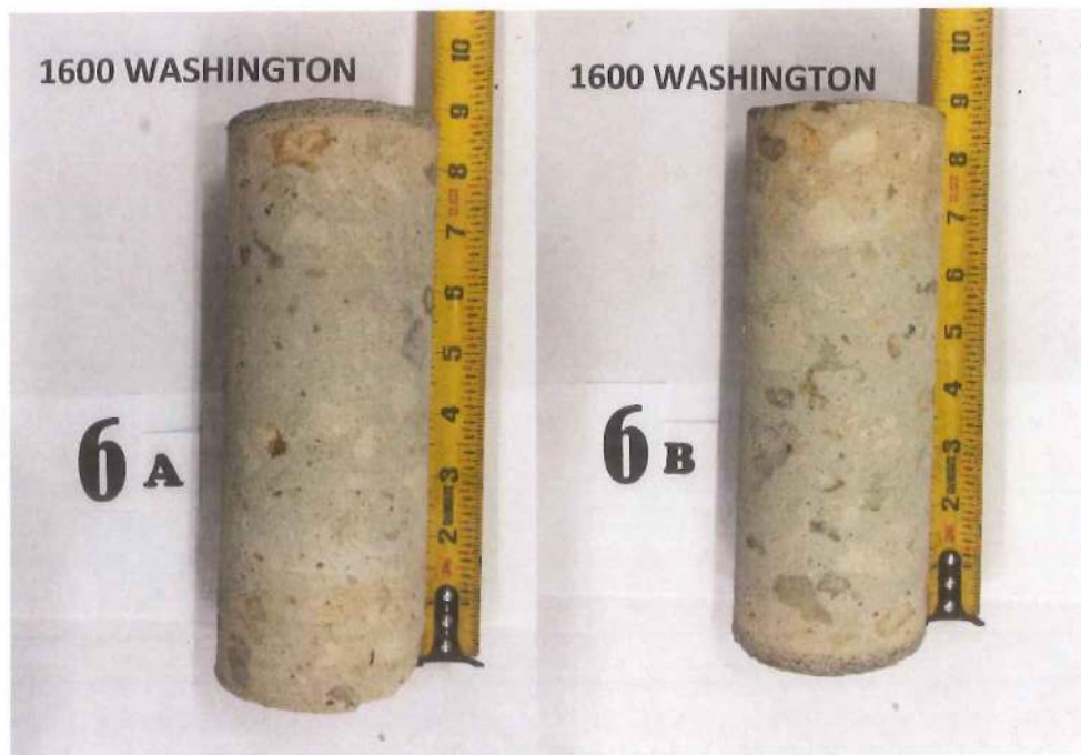
Figure 7: Photograph of Core Samples Level 2 (Compression/Chloride/Carbonation Samples)
