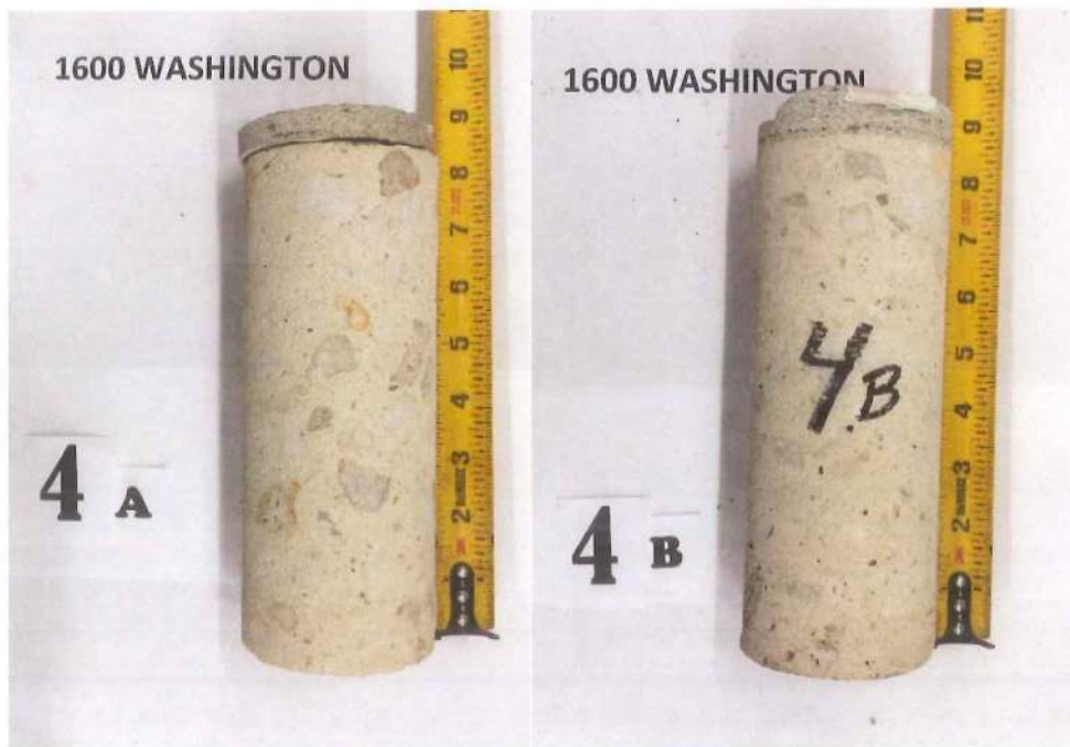
Figure 5: Photograph of Core Samples Level 2 (Compression/Chloride/Carbonation Samples)
