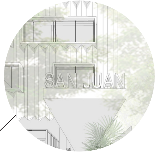
PROJECTING SIGN ON ENTRANCE CANOPY CHANNEL LETTERS - ILLUMINATED 8'-9" W X 1'-8" H - AREA = 15 SF
