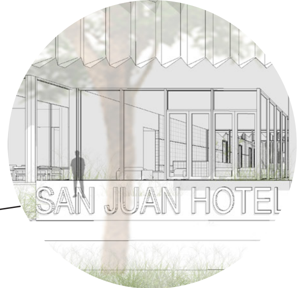
WALL SIGN ON LOW WALL REVERSE CHANNEL LETTERS - ILLUMINATED PIN MOUNTED INDIVIDUAL LETTERS 14'-0" W X 2'-0" H - AREA = 28 SF
