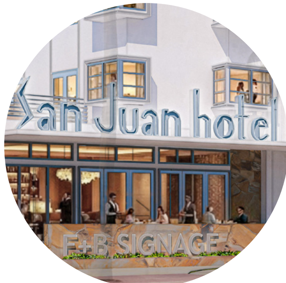
WALL SIGN ON LOW WALL REVERSE CHANNEL LETTERS - ILLUMINATED PIN MOUNTED INDIVIDUAL LETTERS
