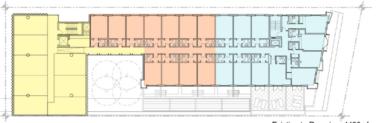
Existing to Remain = 4490 sf Existing to be reconstructed within existing exterior walls = 2730 sf New construction = 2630 sf
