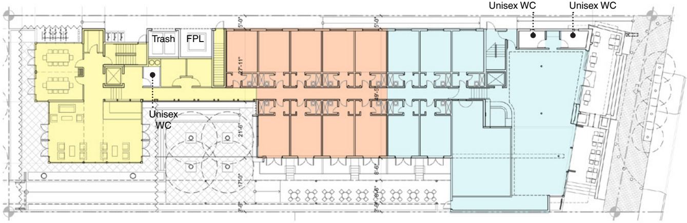
Existing to Remain = 4490 sf Existing to be reconstructed within existing exterior walls = 2730 sf New construction = 2630 sf
