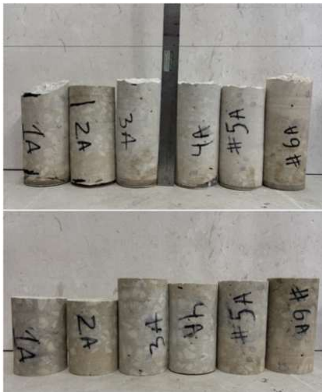
Photograph #2: Concrete Cores Before and After Preparation for Compressive Strength
