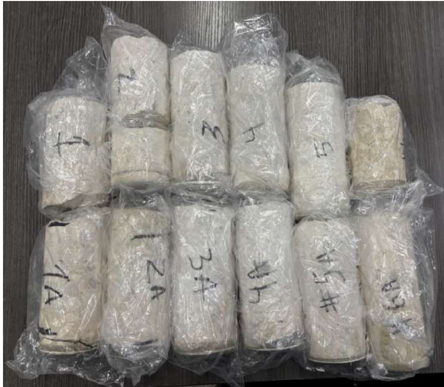
Photograph #1: Concrete Cores Extracted and Bagged for Laboratory Testing
