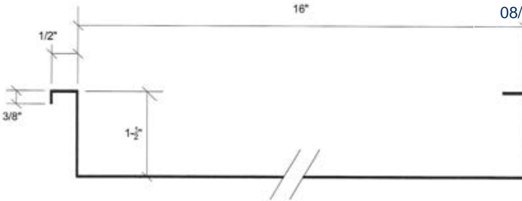
DCM 150 SS - 24GA. STEEL PANEL
