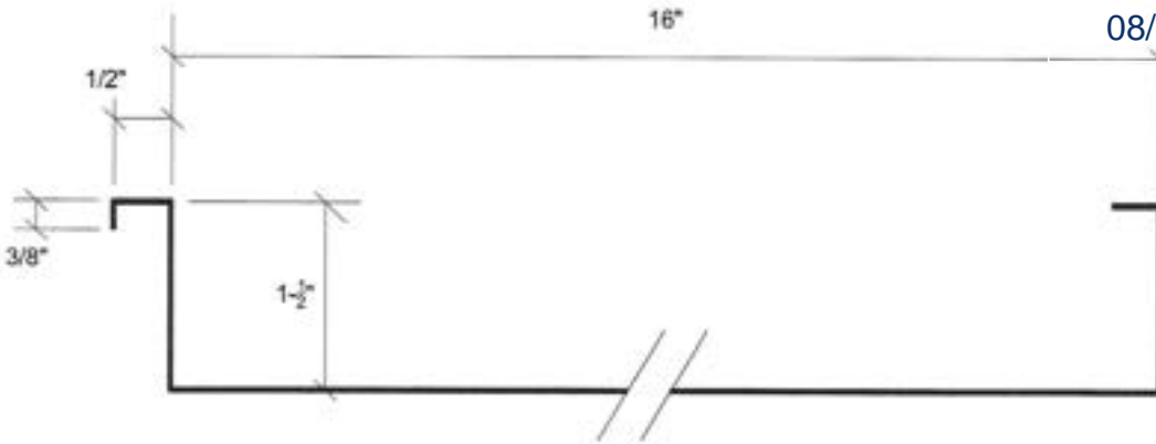
DCM 150 SS - 24GA. STEEL PANEL
