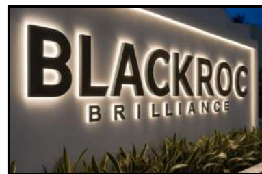
M10 ANODIZED ALUMN. SIGNAGE - BACKLIT
