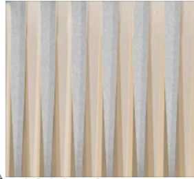
① PROPOSED CUSTOM DECORATIVE METAL CLADDING ON EXISTING PARAPET BY MORRIS ARCHITECTURAL WALL
