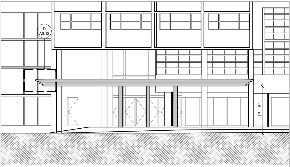
A PROPOSED VALET DROPOFF CANOPY ELEVATION SCALE: 1/16" = 1'-0"
