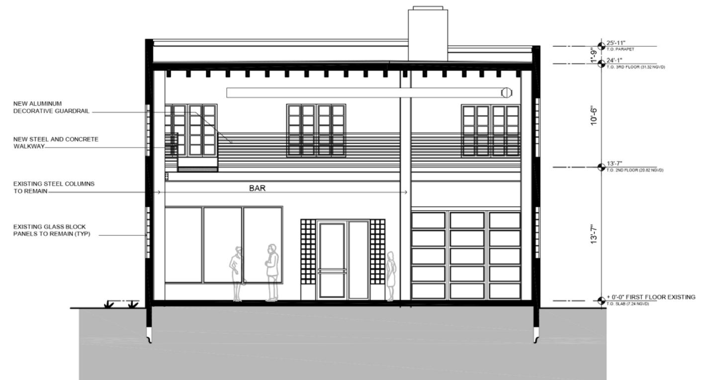
CROSS SECTION LOOKING WEST
