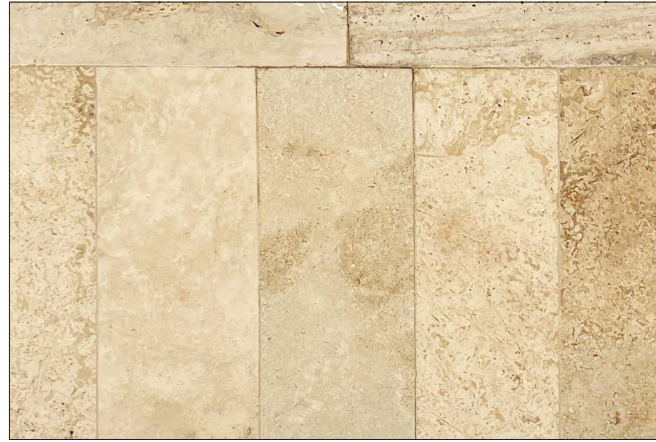
MATERIAL: TRAVERTINE STONE FINISH: SAW CUT, HONED AND FILLED LOCATION: FACADE, CURB AND PLANTER WALL VENEER
