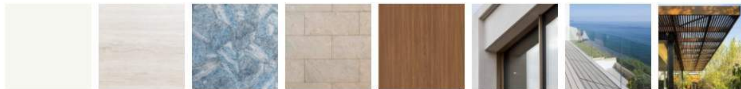
PS-01 PAINTED SMOOTH STUCCO FINISH ST-01 EXTERIOR TILE CLADDING LARGE FORMAT ST-02 EXTERIOR STONE CLADDING LARGE FORMAT ST-03 EXTERIOR TILE CLADDING SMALL FORMAT. WD-01 CLADDED IN SOLID HARDWOOD GL-01 IMPACT GLAZING - CLEAR W/ BRONZE FRAME GLR IMPACT GLASS HANDRAIL - CLEAR WT ALUMINIUM TRELLIS CLADDED IN WOOD
