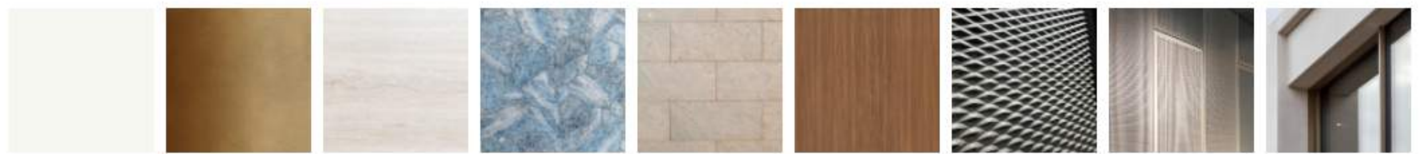
PS-01 PAINTED SMOOTH STUCCO FINISH MT-01 METAL COLUMN COVER, BRUSHED BRONZE ALUMINIUM FINISH ST-01 EXTERIOR TILE CLADDING LARGE FORMAT ST-02 EXTERIOR STONE CLADDING LARGE FORMAT ST-03 EXTERIOR TILE CLADDING SMALL FORMAT. WD-01 CLADDED IN SOLID HARDWOOD MS-01 ALUMINIUM MECHANICAL SCREEN MS-02 METAL SCREEN GL-01 IMPACT GLAZING - CLEAR W/ BRONZE FRAME
