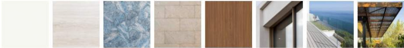
PS-01 PAINTED SMOOTH STUCCO FINISH ST-01 EXTERIOR TILE CLADDING LARGE FORMAT ST-02 EXTERIOR STONE CLADDING LARGE FORMAT ST-03 EXTERIOR TILE CLADDING SMALL FORMAT. WD-01 CLADDEN IN SOLID HARDWOOD GL-01 IMPACT GLAZING - CLEAR W/ BRONZE FRAME GLR IMPACT GLASS HANDRAIL - CLEAR WT ALUMINIUM TRELLIS CLADDEN IN WOOD
