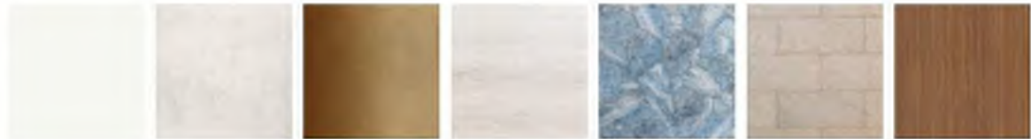
PS-01 PAINTED SMOOTH STUCCO FINISH VP-01 VENETIAN PLASTER FINISH MT-01 METAL COLUMN COVER, BRUSHED BRONZE ALUMINIUM FINISH ST-01 EXTERIOR TILE CLADDING LARGE FORMAT ST-02 EXTERIOR STONE CLADDING LARGE FORMAT ST-03 EXTERIOR TILE CLADDING SMALL FORMAT. WD-01 CLADDED IN SOLID HARDWOOD
