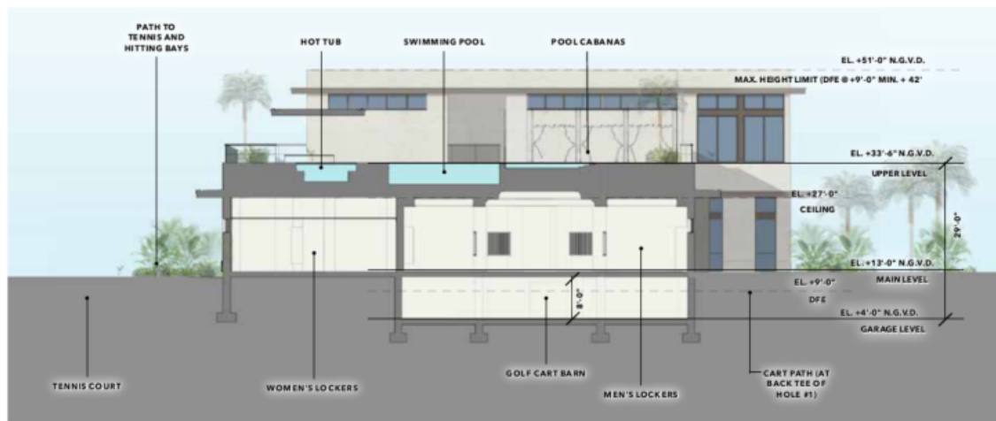
SECTION THROUGH WELLNESS BUILDING E-W
