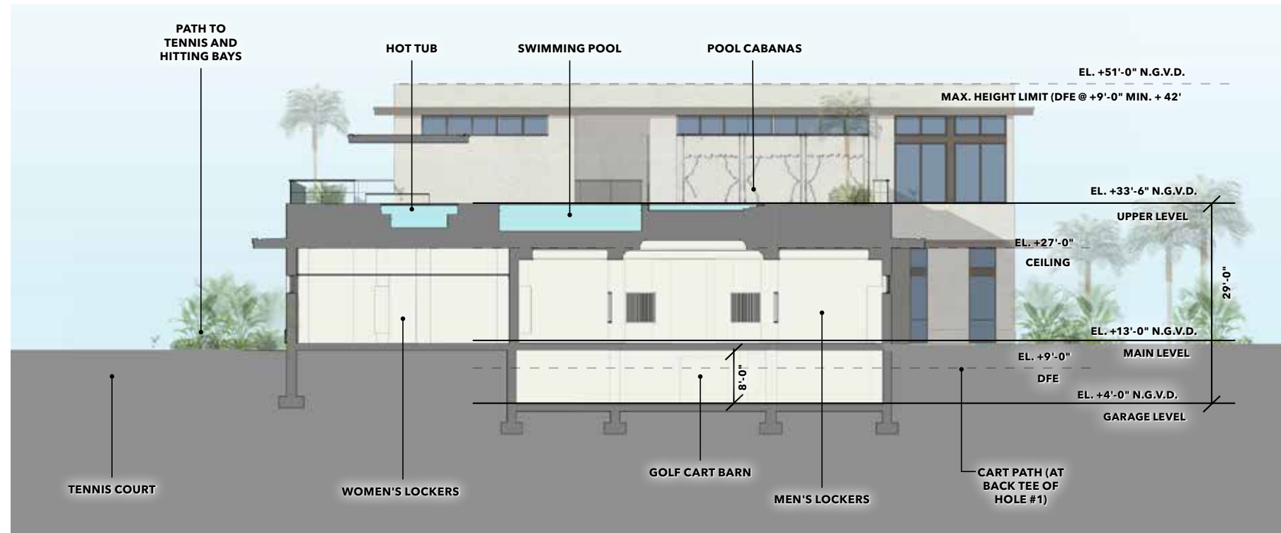
SECTION THROUGH WELLNESS BUILDING E-W
