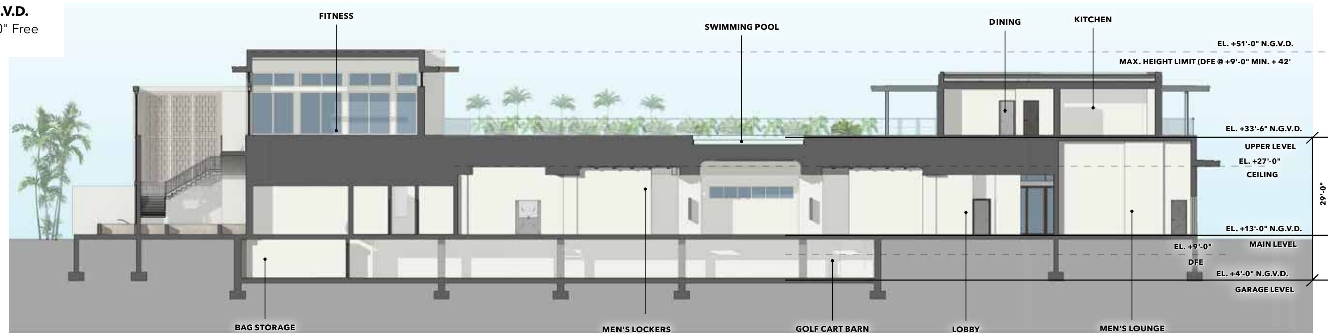
SECTION THROUGH WELLNESS BUILDING N-S
