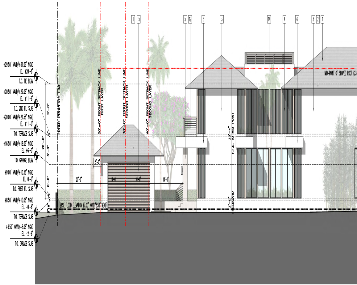
1 LOT 9 - WEST ELEVATION (PARTIAL) A1.0/A5.2 3/20' = 1'-0"
