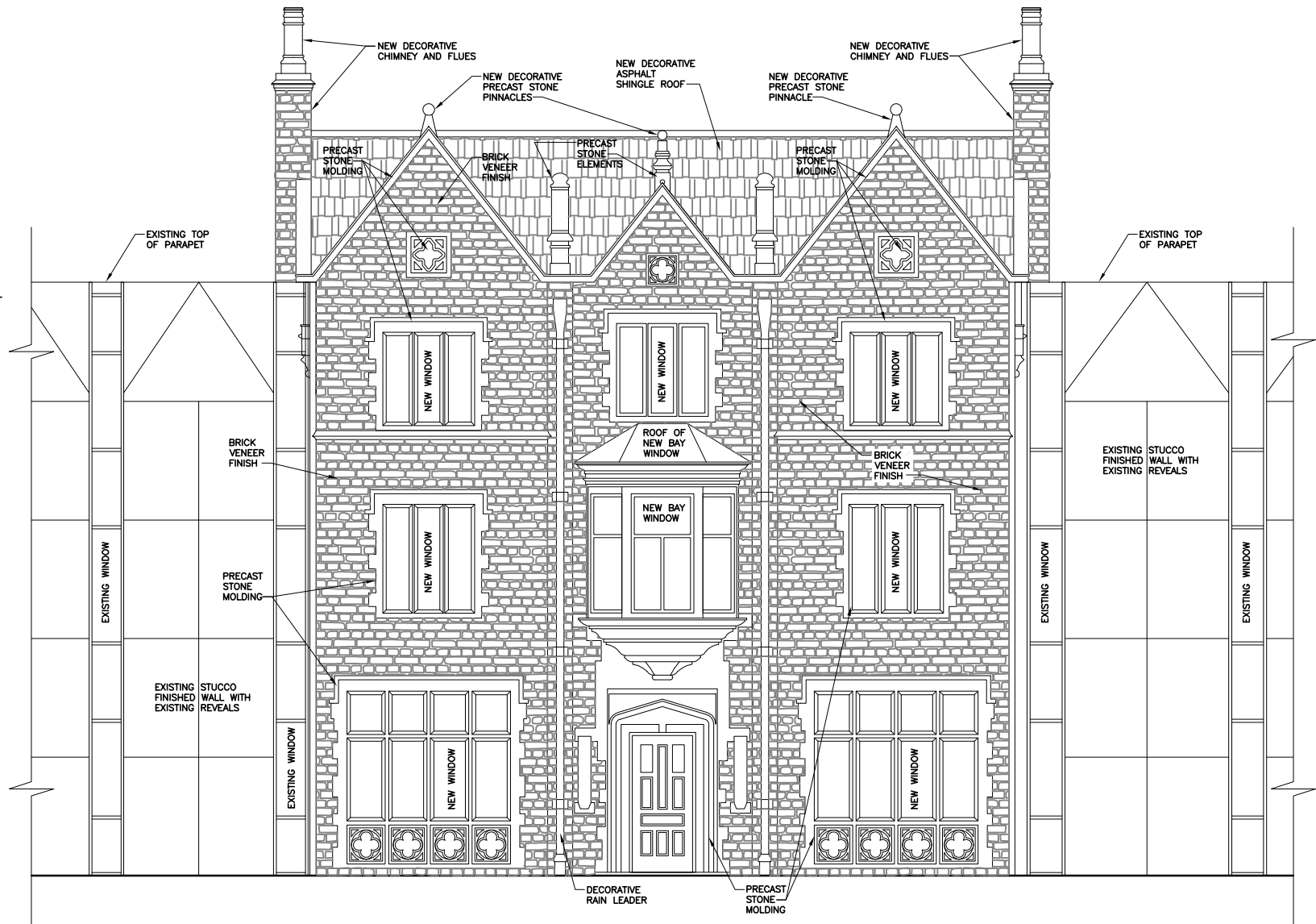
FRONT FACADE ELEVATION 1 SCALE: 1/8" = 1'-0"
