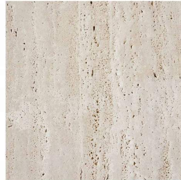
STN 1 TRAVERTINE CLADDING
