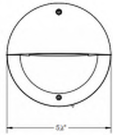
⑦ RECESSED SCNCE @ HISTORICAL BUILDING AND STUCCO WALLS AT SIDEWALK. NOTE STUCCO WALLS AT SIDEWALK HAS 3/4" DEEP NICHE. OUTER EDGE OF SCNCE ALIGNS WITH OUTER EDGE OF WALLS.
