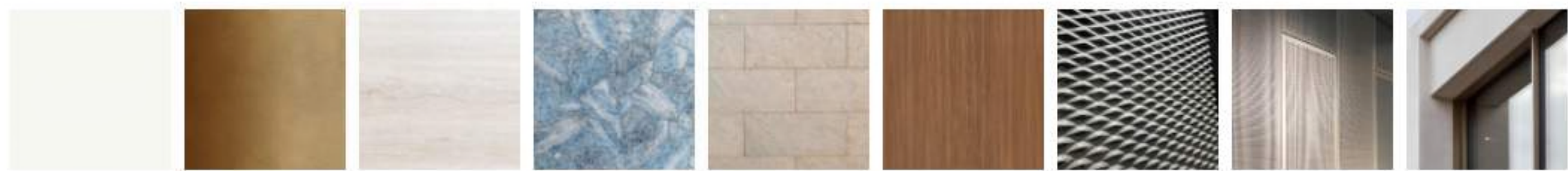
PS-01 PAINTED SMOOTH STUCCO FINISH MT-01 METAL COLUMN COVER, BRUSHED BRONZE ALUMINIUM FINISH ST-01 EXTERIOR TILE CLADDING LARGE FORMAT ST-02 EXTERIOR STONE CLADDING LARGE FORMAT ST-03 EXTERIOR TILE CLADDING SMALL FORMAT. WD-01 CLADDEN IN SOLID HARDWOOD MS-01 ALUMINIUM MECHANICAL SCREEN MS-02 METAL SCREEN GL-01 IMPACT GLAZING - CLEAR W/ BRONZE FRAME
