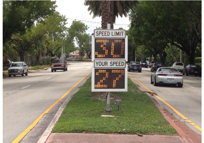
Digital speed readout signs remind motorists when they are exceeding the speed limit along Alton Road.
