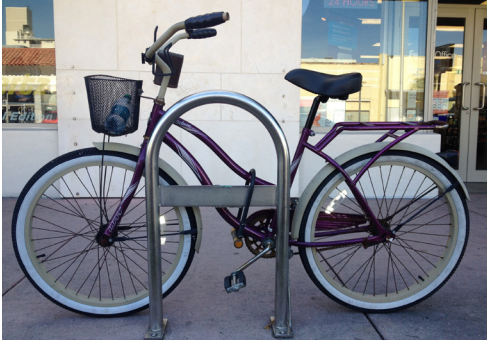
A INVERTED U-RACK (RECOMMENDED)
