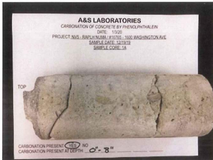
Figure 8: Carbonation Core Sample No. 1A: Level 1 Column
