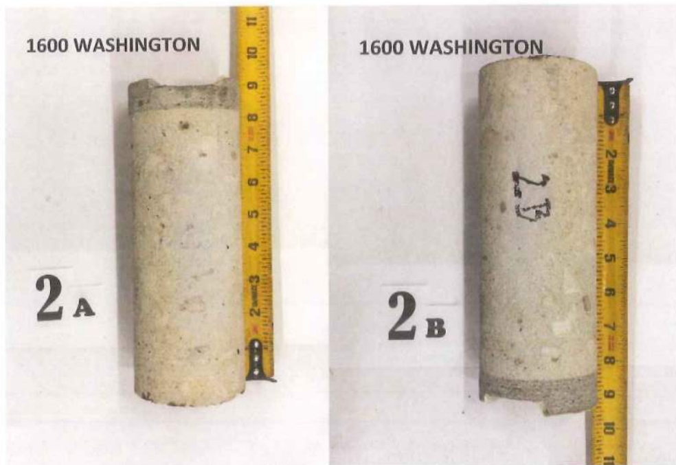
Figure 3: Photograph of Core Samples Level 1 Column (Compression/Chloride/Carbonation Samples)
