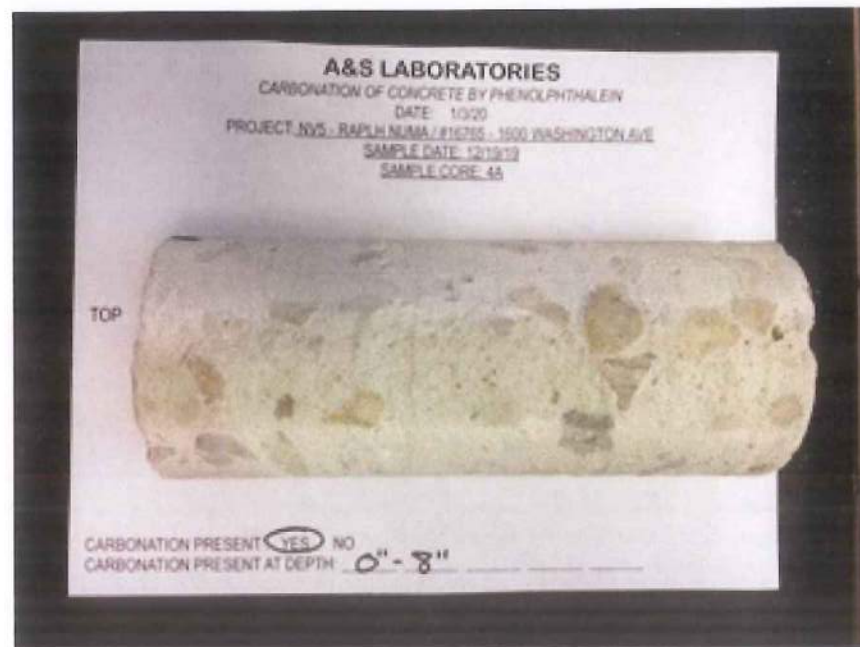
Figure 11: Photograph Core Sample No. 4A: Level 2 Column
