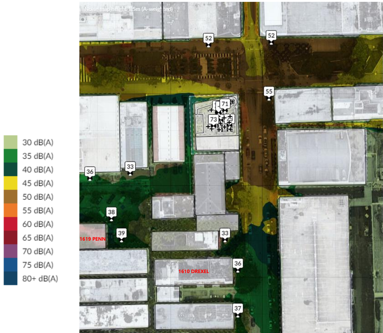
Figure 6 - dBMap View showing sound projected 5 ft. above the ground. The receiver points are L_{smax} dBA sound pressure level.
