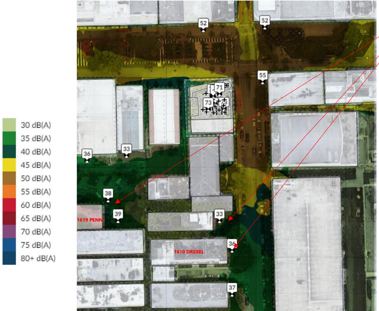
Figure 6 - dBMap View showing sound projected 5 ft. above the ground. The receiver points are Lsmax dBA sound pressure level.
