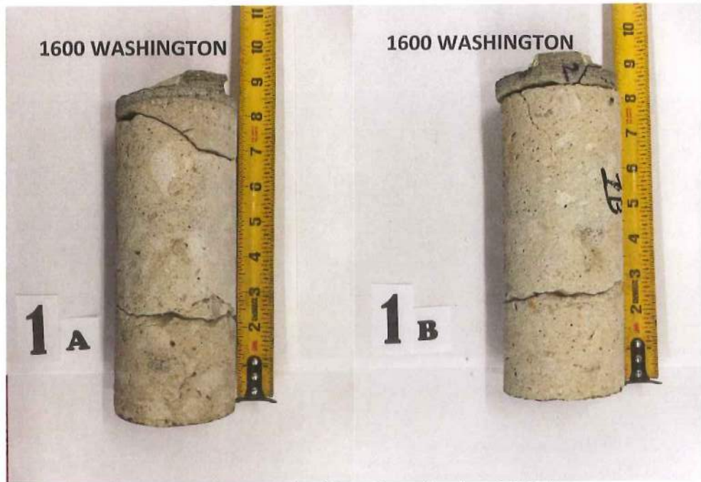
Figure 2: Photograph of Core Samples Level 1 Column (Compression/Chloride/Carbonation Samples)
