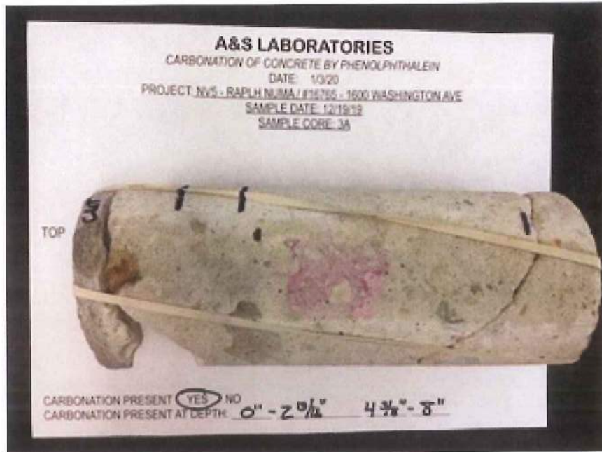
Figure 10: Photograph Core Sample No. 3A: Level 1 Column
