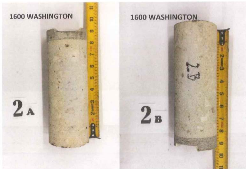
Figure 3: Photograph of Core Samples Level 1 Column (Compression/Chloride/Carbonation Samples)
