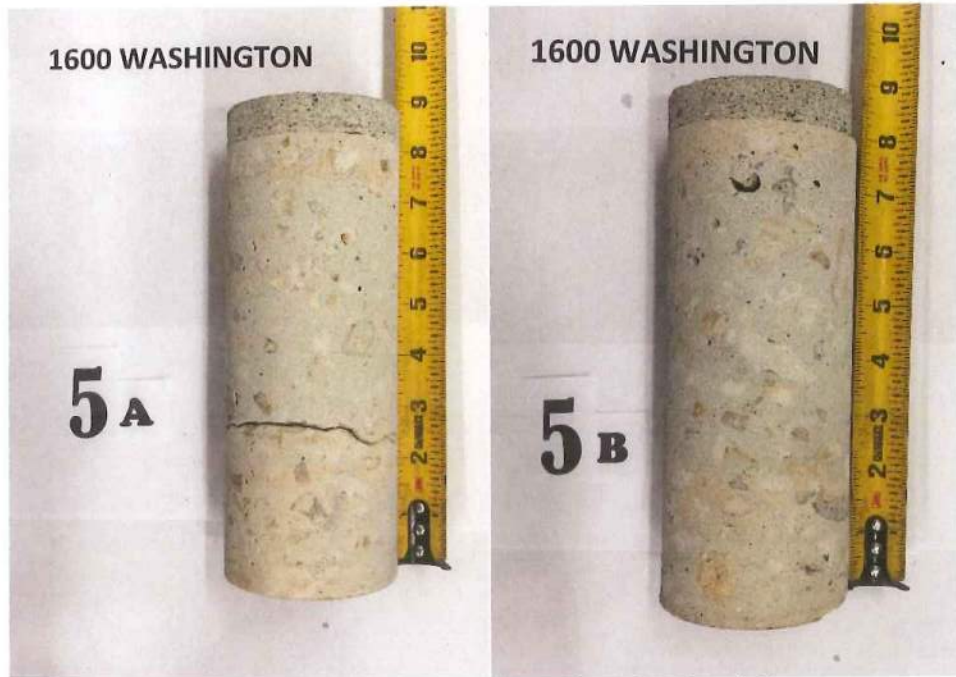
Figure 6: Photograph of Core Samples Level 2 (Compression/Chloride/Carbonation Samples)
