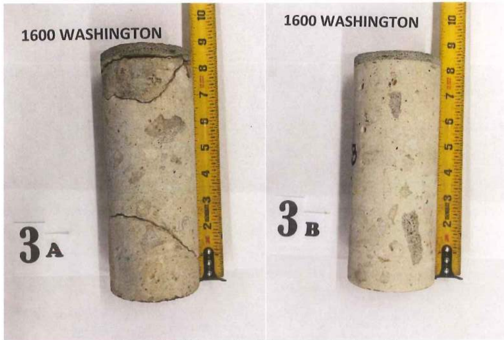
Figure 4: Photograph of Core Samples Level 1 (Compression/Chloride/Carbonation Samples)
