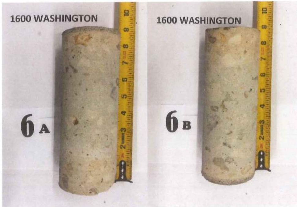
Figure 7: Photograph of Core Samples Level 2 (Compression/Chloride/Carbonation Samples)
