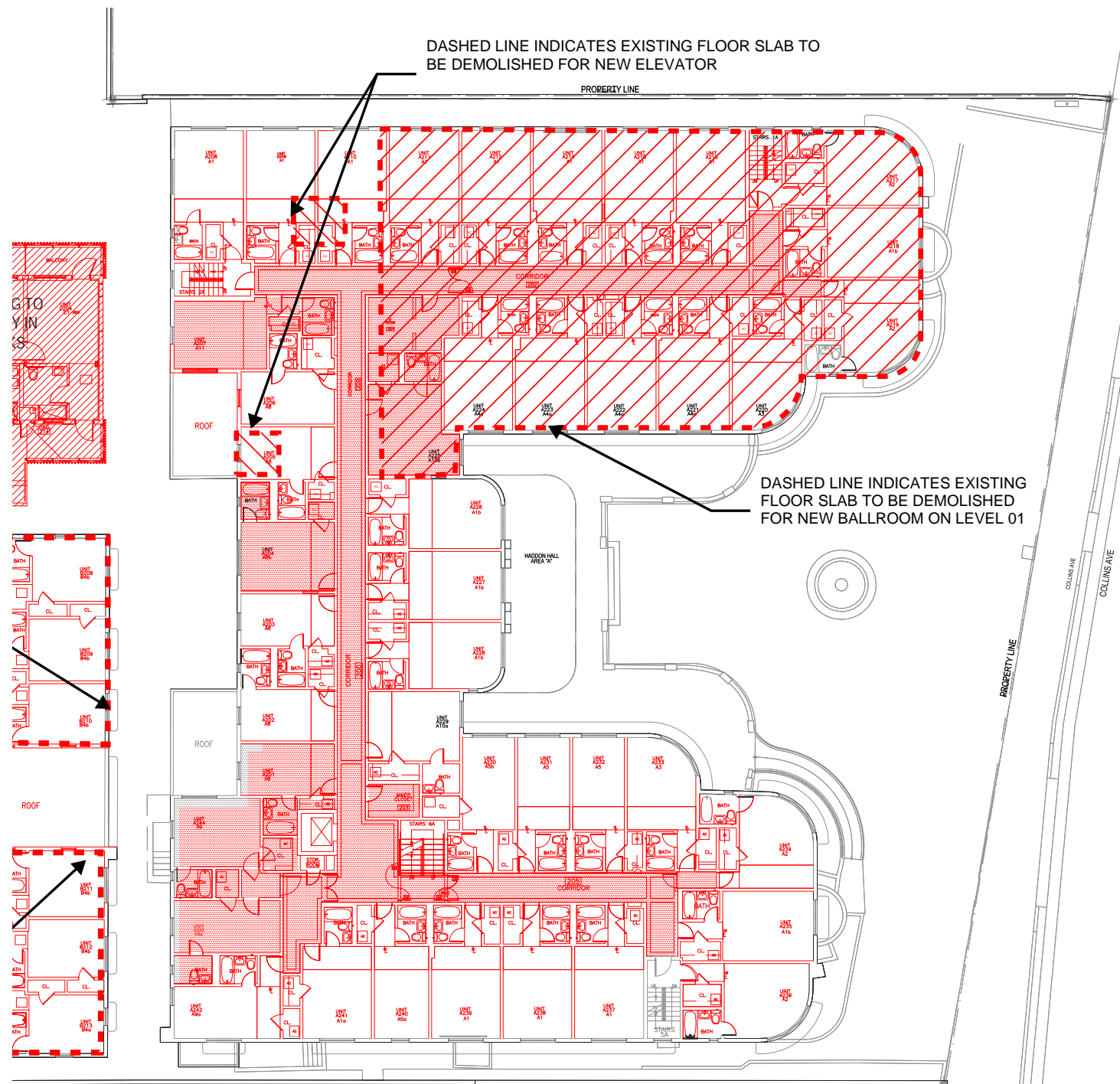
LEVEL 02: DEMOLITION PLAN
