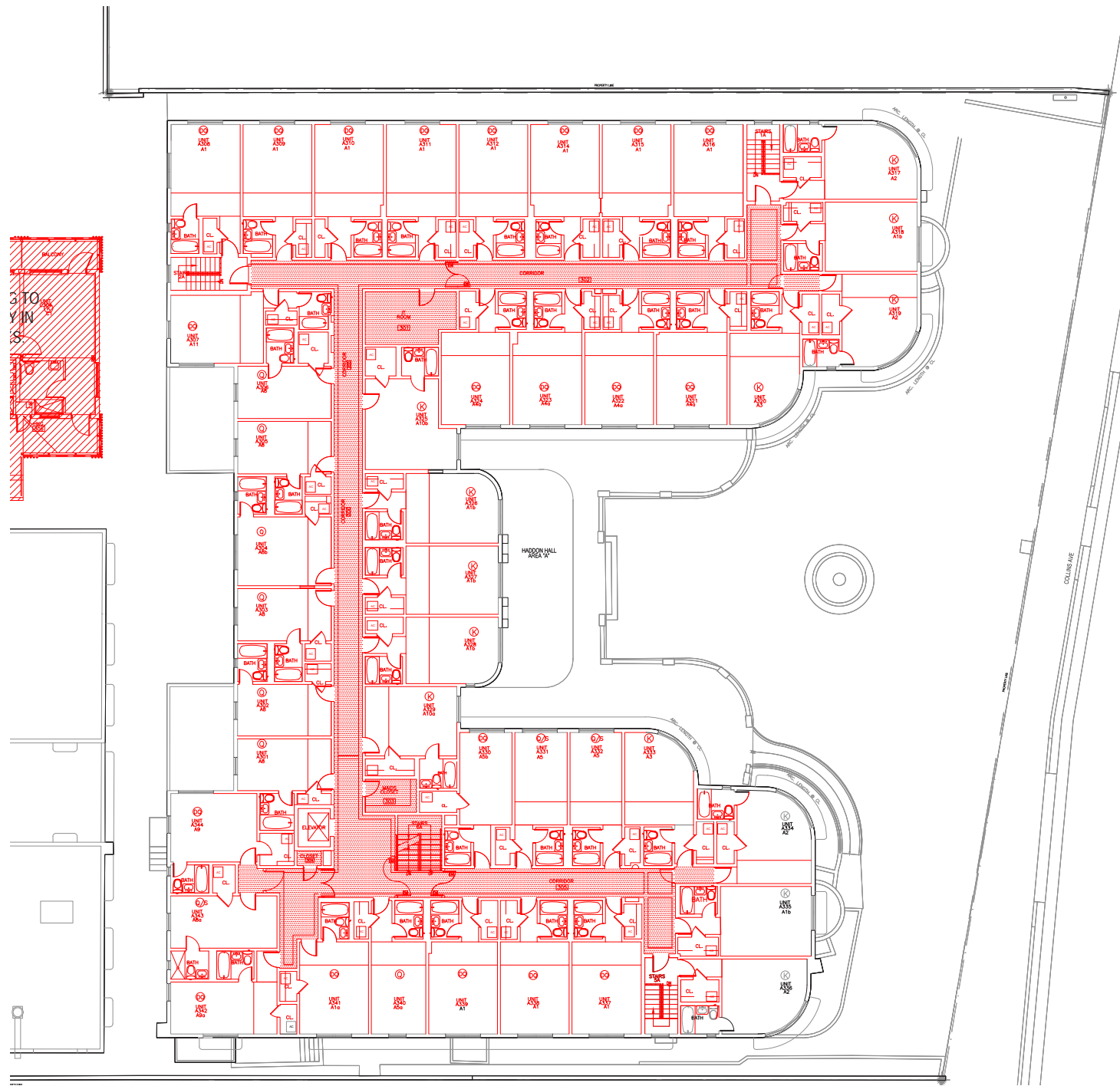
LEVEL 03: DEMOLITION PLAN
