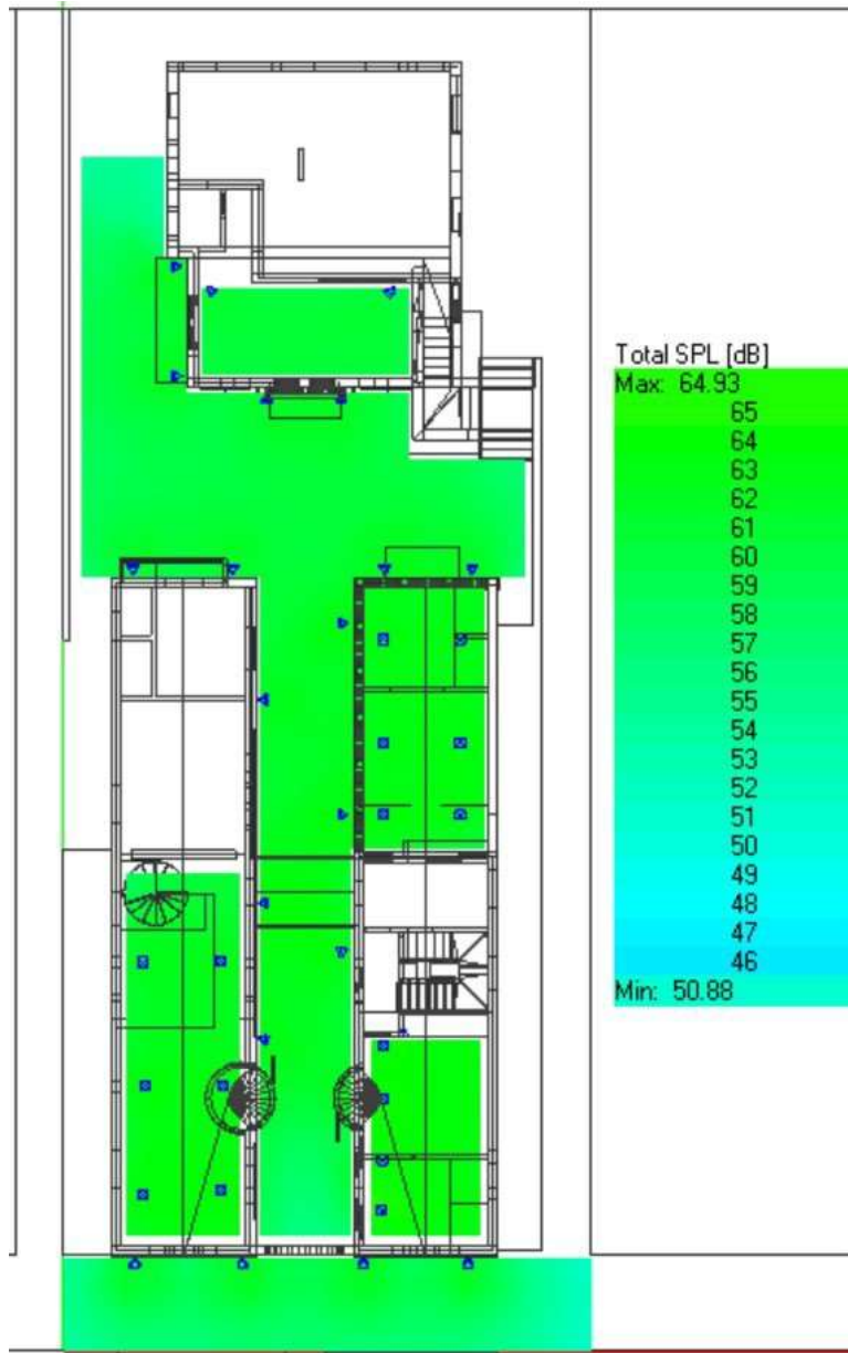
Sound Pressure Level MAP in dBA - 65 dBA max (plan view)
