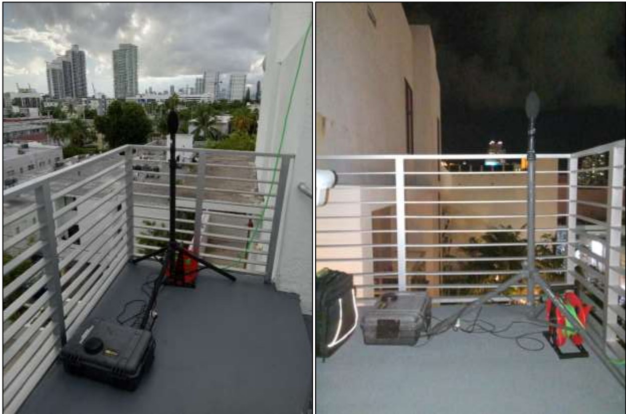
Figures 2 and 3: Monitoring system and microphone at measurement location.
