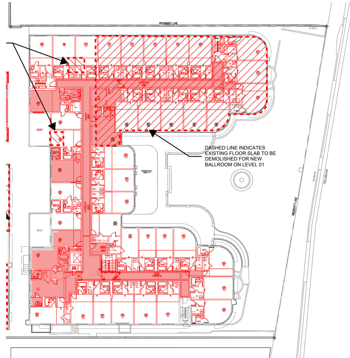
LEVEL 02: DEMOLITION PLAN
