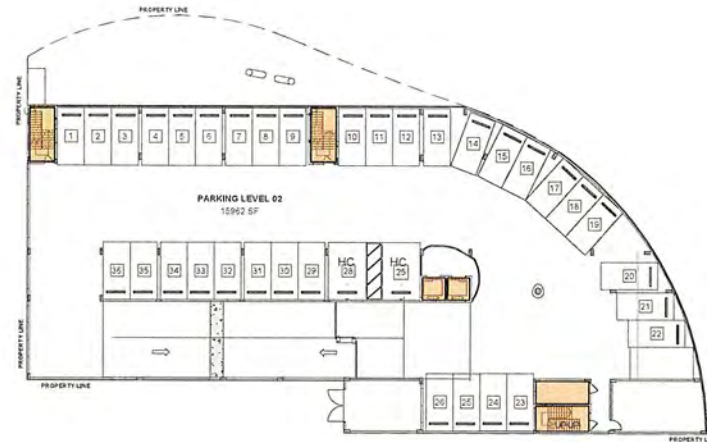
2 2ND FLOOR F.A.R. DIAGRAM TOTAL F.A.R. LEVEL 02 - 623.97 SF SCALE: 3/16" = 1'-0"
