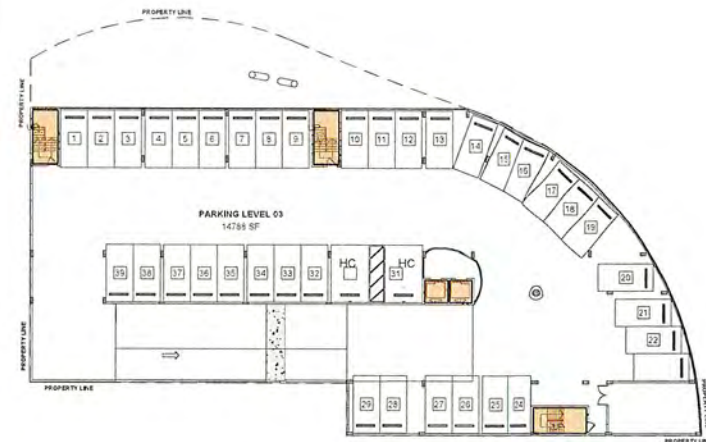
3 3TH FLOOR F.A.R. DIAGRAM TOTAL F.A.R. LEVEL 03 - 505.14 SF SCALE: 3/16" = 1'-0"
