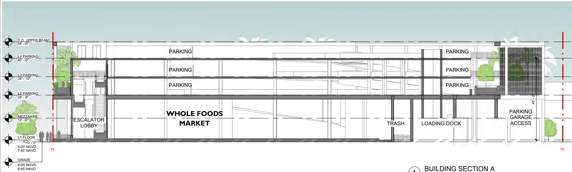
① BUILDING SECTION A 3/64" = 1'-0"
