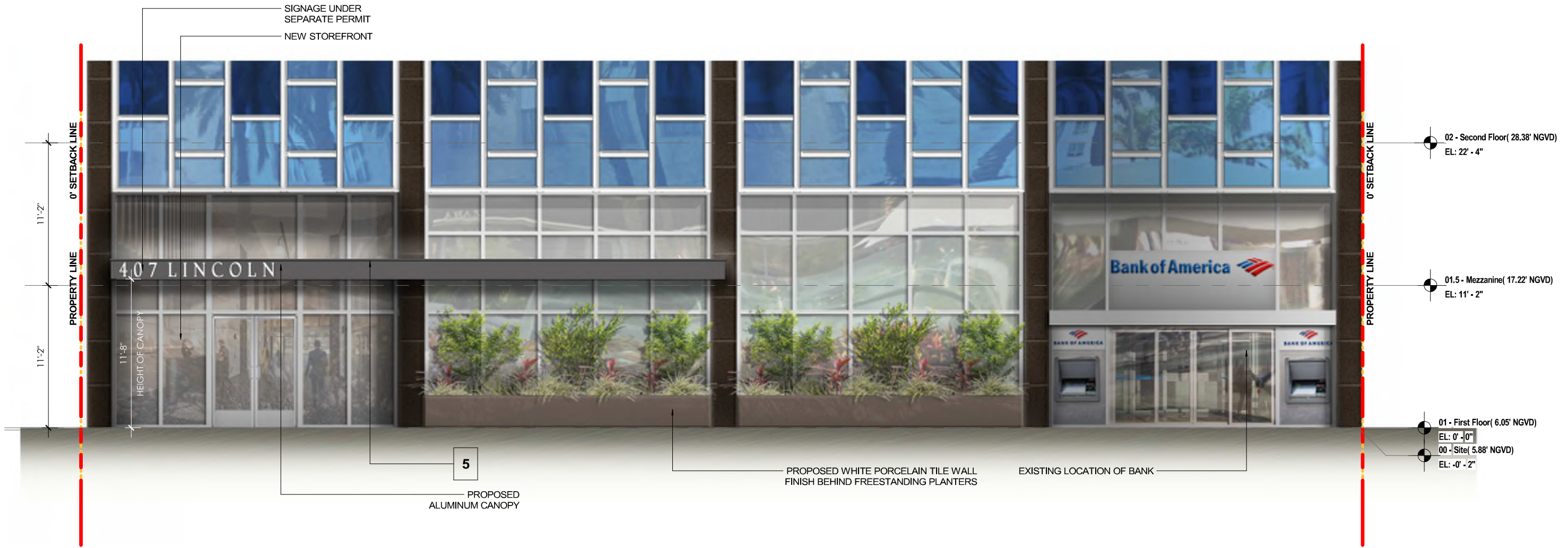
1 Proposed - Enlarged Elevation @ Exterior Front Canopy-Rendered A-31.0 Scale: 1/8" = 1'-0"
