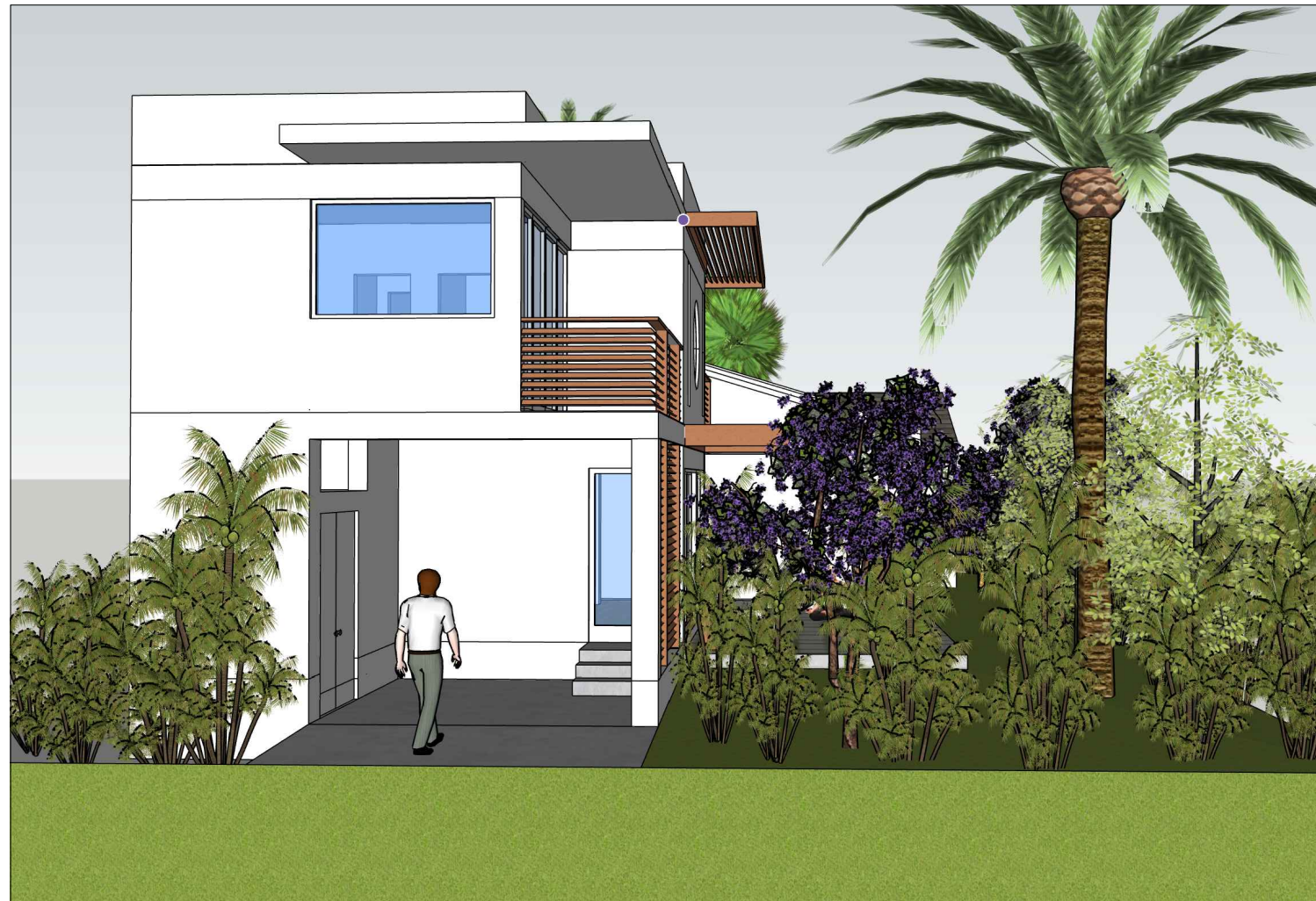
West elevation of proposed addition showing south facing louvered wood sunscreens and balcony rail.
