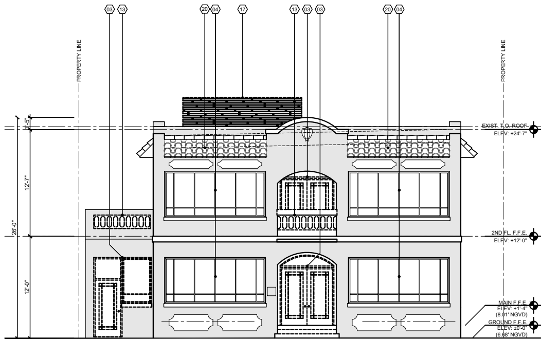
EXIST. / DEMO EAST ELEVATION SCALE: 3/16" = 1'-0"
