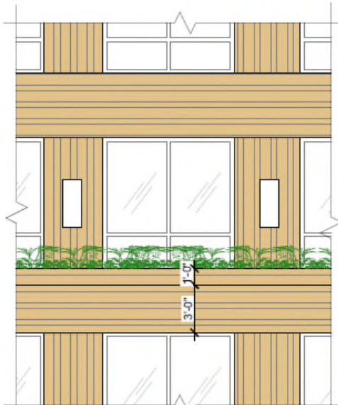
2 PROPOSED BALCONY ENLARGED ELEVATION SCALE: 1/4"
