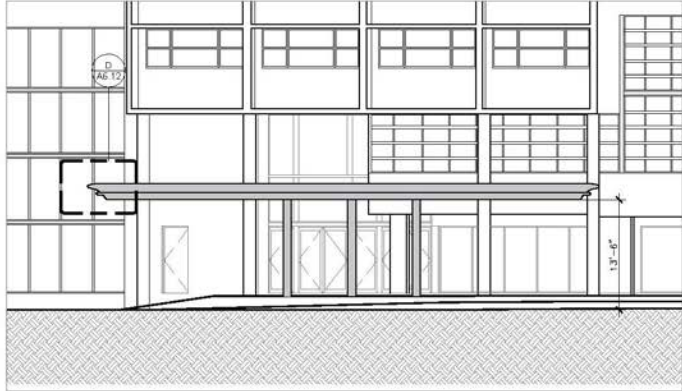
A PROPOSED VALET DROPOFF CANOPY ELEVATION SCALE: 1/16" = 1'-0"
