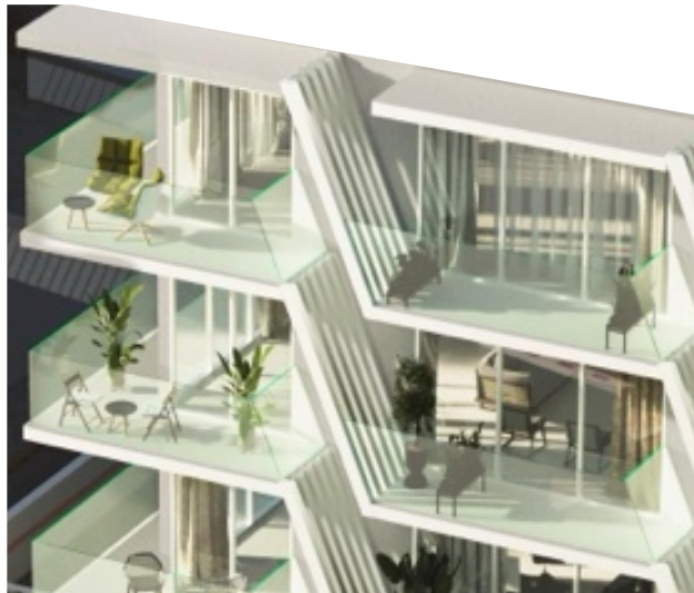
12 SLANTED ALUMINUM BALCONY LOUVERS
