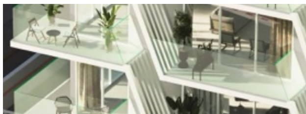
12 SLANTED ALUMINUM BALCONY LOUVERS
