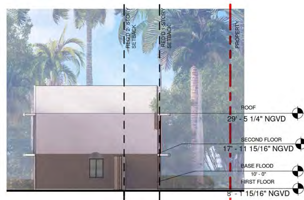
2 BUILDING 4 PROPOSED SOUTH ELEVATION. 1/16" = 1'-0"
