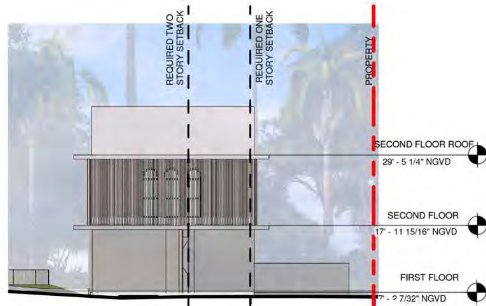
3 BUILDING 5 PROPOSED SOUTH ELEVATION 1/16" = 1'-0"
