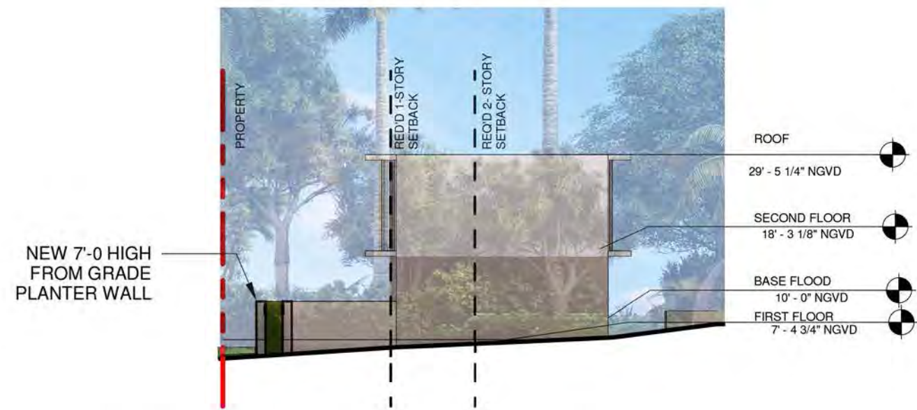
4 BUILDING 5 PROPOSED NORTH ELEVATION 1/16" = 1'-0"
