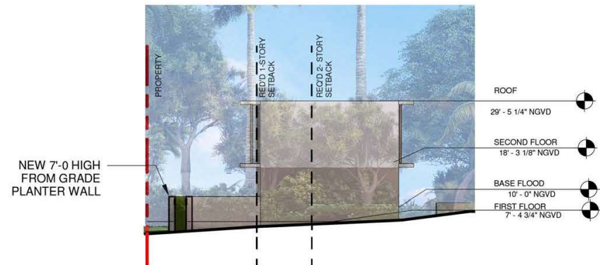
4 BUILDING 5 PROPOSED NORTH ELEVATION 1/16" = 1'-0"
