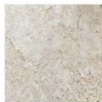
ST2 STONE CLADDING: ROUGH FACE
