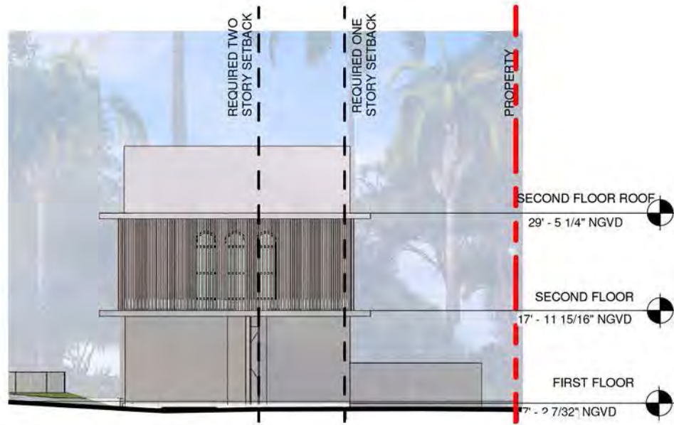
3 BUILDING 5 PROPOSED SOUTH ELEVATION 1/16" = 1'-0"
