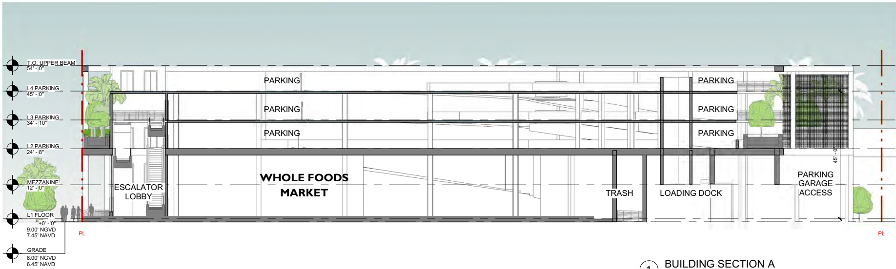
① BUILDING SECTION A 3/64" = 1'-0"
