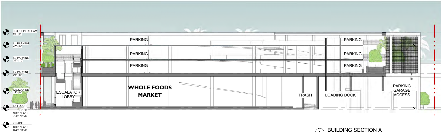
① BUILDING SECTION A 3/64" = 1'-0"
